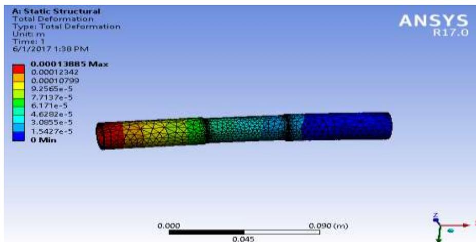
**Fig 7.1 – Figure Showing Deformation Of Al-Alloy**
