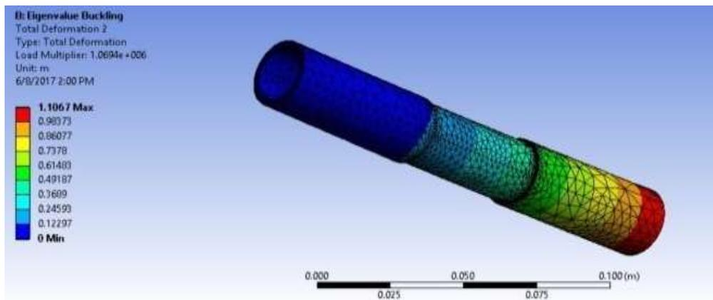
Fig 7.4 – Figure Showing Buckling Results For Al-Alloy
