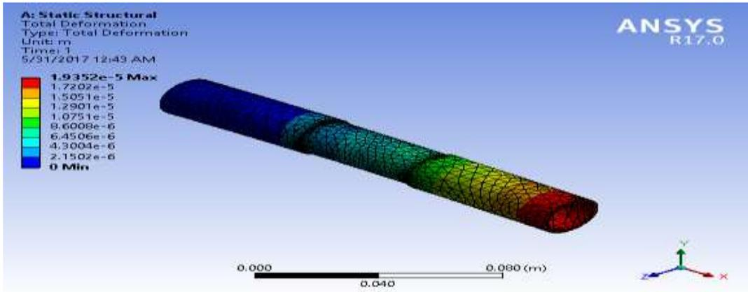
Fig 7.2 –Figure Showing Deformation Of HS Carbon/Epoxy (0/30/45/60/90)S
