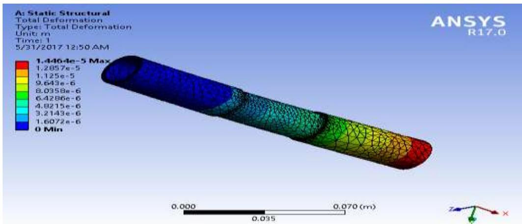
Fig 7.3 –Figure Showing Deformation Of HM Carbon/Epoxy (0/30/45/60/90)S
