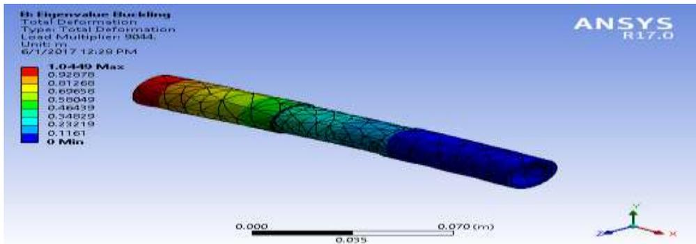
Fig 7.6 – Figure Showing Buckling Results For HM Carbon/Epoxy(0/30/45/60/90)S
